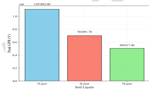
Figure 6. GPR peak bar graph in desert areas and summer season for horizontal soil models uniform , two-layer and three-layer
