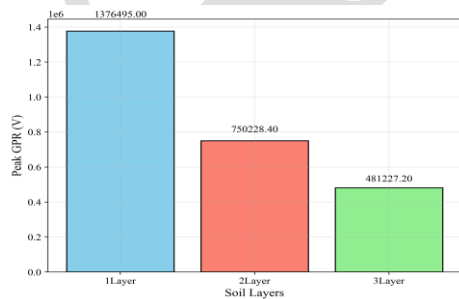
Figure 18. GPR peak bar graph in mountainous areas and summer season for horizontal soil models uniform, two-layer and three-layer
